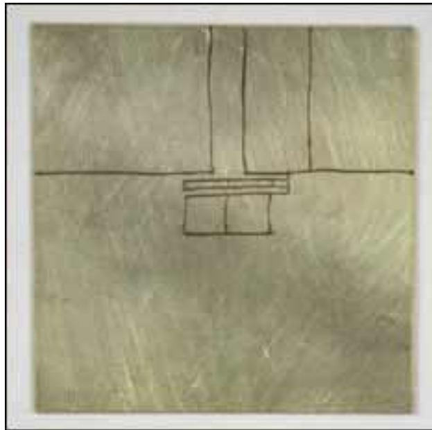
Figure 4. The cut circuit board, made using copper-clad and a roto-tool, realizes the layout drawing of Figure 2.
